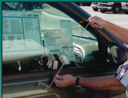
7. Wedge open the weather-stripping near the center of the front door.
